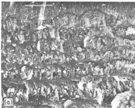
Figure 4 Fracture surface of the knee region shown in Fig. 3. In both pictures the white bar at the top left represents 25 \mu\text{m} . (a) The outer part of the knee, at the outer surface is at the top. (b) The inner, less highly calcified region.
